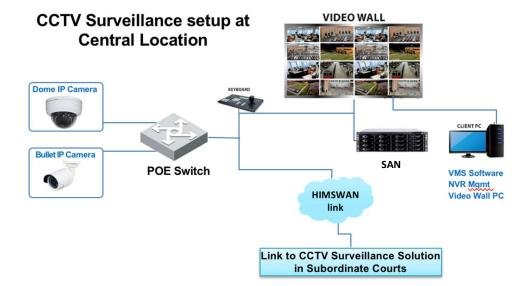
The overall architecture for CCTV Surveillance at Central Location would be as follows:
