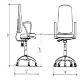
ARMREST ASSEMBLY: The one-piece armrests should be injection moulded from black Nylon. The armrests should be fitted to the seat with armrest connecting brackets made of 0.5  $\pm$  0.05 cm. Thick HR steel.
