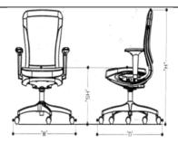
PNEUMATIC HEIGHT ADJUSTMENT: The seating height can be adjusted with a pneumatic gas-lift having an adjustment stroke of  $9.2 \pm 0.3$  cm.
