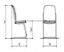
The seat and back are made up of  $1.2\pm0.1$ cm. Thick hot-pressed plywood measured. Upholstered with fabric upholstery covers and moulded Polyurethane foam. The back foam is designed with contoured lumbar support for extra comfort. The seat has extra thick foam on front edge to give comfort to popliteal area. MID BACK SIZE 47.5 cm. (W) x 58.0 cm. (H). SEAT SIZE 47.0 cm. (W) x 48.0 cm. (D)
