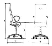
TWIN WHEEL CASTORS: The twin wheel castors are injection moulded in Black Nylon.
